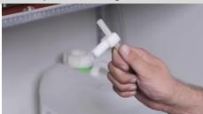
Open the cap of the full cartridge using the barrel wrench (this is included in the accessories of your Ecoport) by turning it counterclockwise
