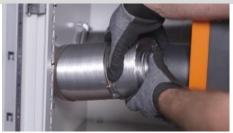
Attach the inner corrugated aluminum pipe ( $\emptyset$  70 mm) to the inner exhaust pipe of the Ecoport and fix it with the pipe clamp ( $\emptyset$  70 mm)
