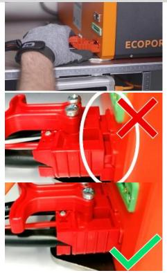
Insert the battery cable into the battery plug of the Ecoport.
