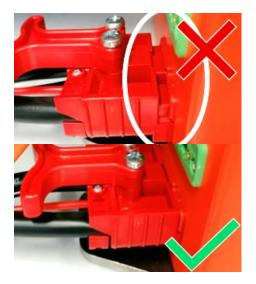
Description: The Ecoport does not perform a function check (start the fans) after connecting the battery and the signal light on the control panel does not light up.
