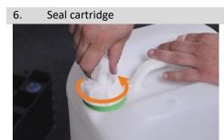
Close the old cartridge with a sealing cap and hand-tighten it with the barrel wrench by turning it clockwise.
