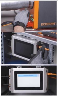
Use the data cable (Ethernet RJ-45) included in the accessories to connect the Ecoport to the control panel.
