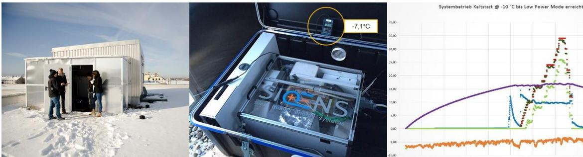
In January 2016, Sicens proved under real-life conditions that its fuel cell system is not damaged in any way by being frozen. In a field test, the system was put back into operation after it was fully frozen overnight – its restart was flawless. In contrast to several competing products, freezing a Sicens fuel cell is a noncritical process, which – since the system does not need to be kept warm unnecessarily – reduces operating costs and makes winter transports a breeze.
